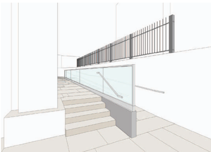
Top, sketch render of external ramp offering disabled access and additional entry point into the building along eastern elevation.
